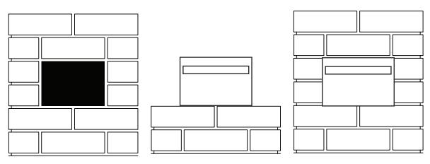
SLEEVE FITS INTO 1 BRICK WIDE BY 2 BRICK HIGH CAVITY Build up brickwork to desired height and set letterbox in place
